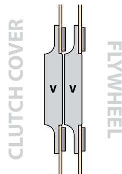
V = Solid, 8 rivet, outer (.375" thick)
