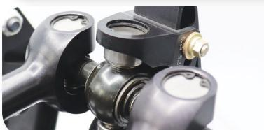
*Pedal pivots feature needle bearing and/or ball bearings for the ultimate in smooth operation and service life.*
