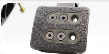
*Adjustable clutch and/or throttle stops limit pedal travel (most models).*
